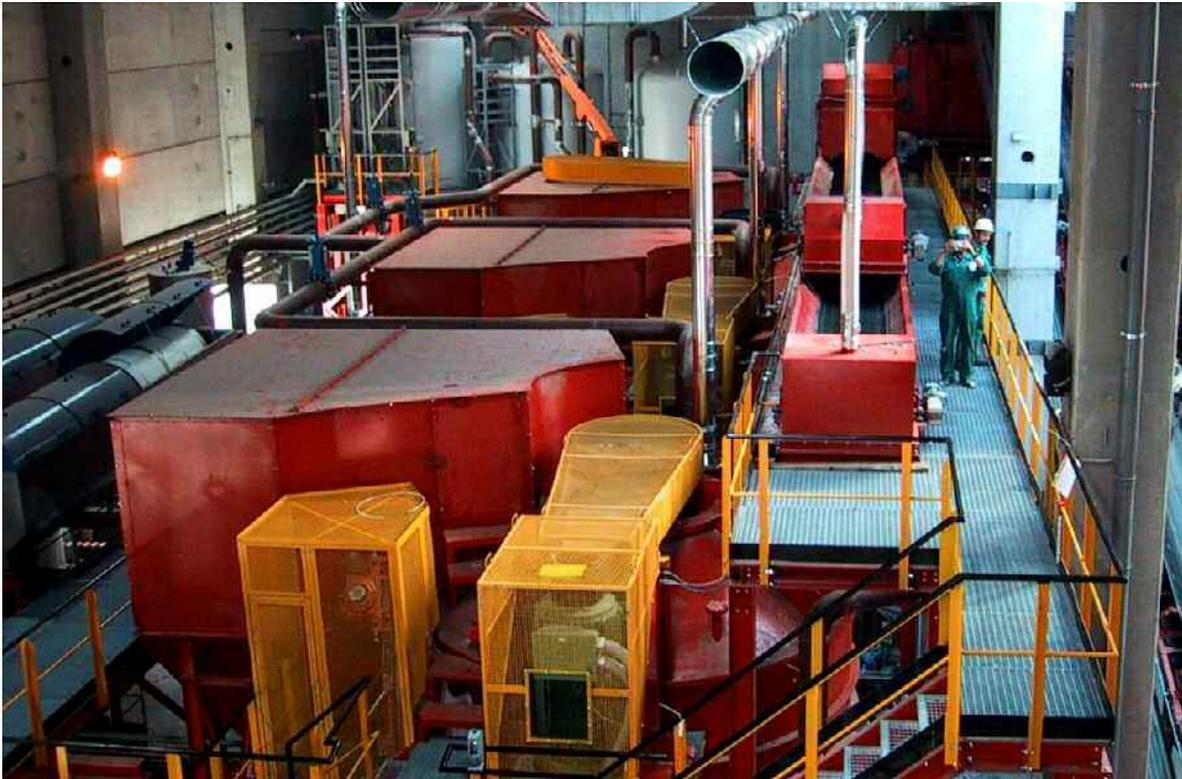
**Figure 4** Wet-mechanical BTA processing in Ca' del Bue, Verona – left edge: thickening, in the background: BTA grit removal system
