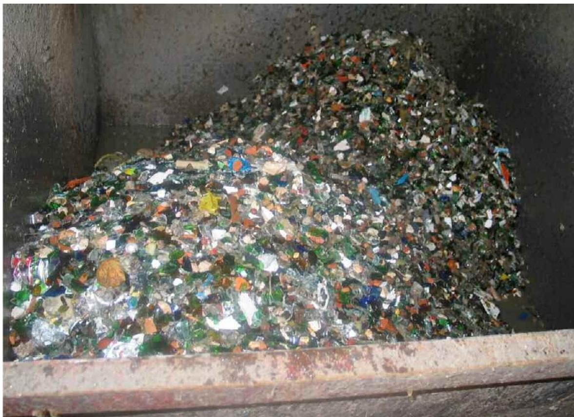
**Figure 7** Separated heavy fraction of the wet-mechanical processing
